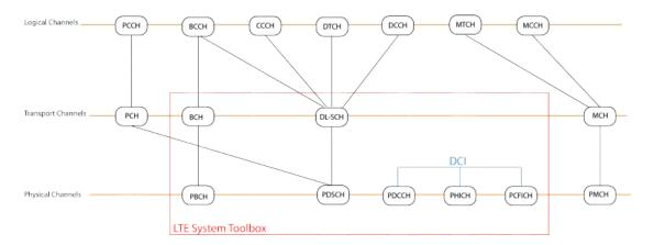
The LTE System Toolbox product offers functionality for the downlink physical channels, transport channels, and control information outlined in red in the preceding figure. For more information, see the following categories.
