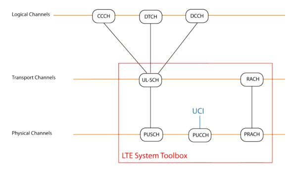
The LTE System Toolbox product offers functionality for the uplink physical channels, transport channels, and control information outlined in red in the preceding figure. For more information, see the following categories.
